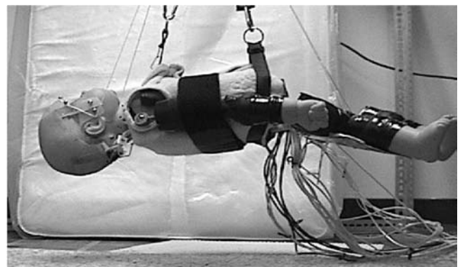
FIG. 5. Photograph representing a worst-case scenario. The surrogate was suspended and released in a supine position with legs extended and arms fixed to the torso. This configuration resulted in initial ground contact to occur with the head of the surrogate.
